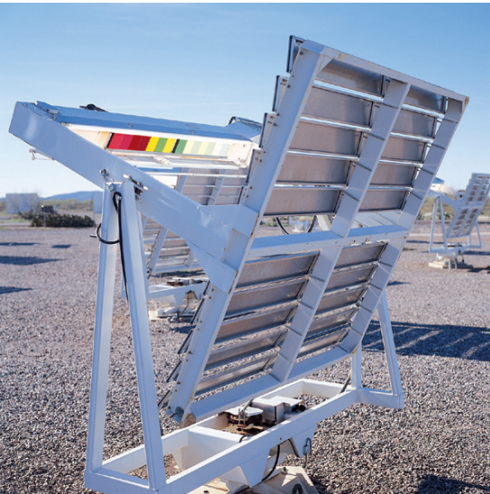
The RENOLIT ALKORTEC roofing membrane is tested for ageing in some of the harshest environments on the planet: in Florida (humid tropical climate) and in Arizona (desert climate).
