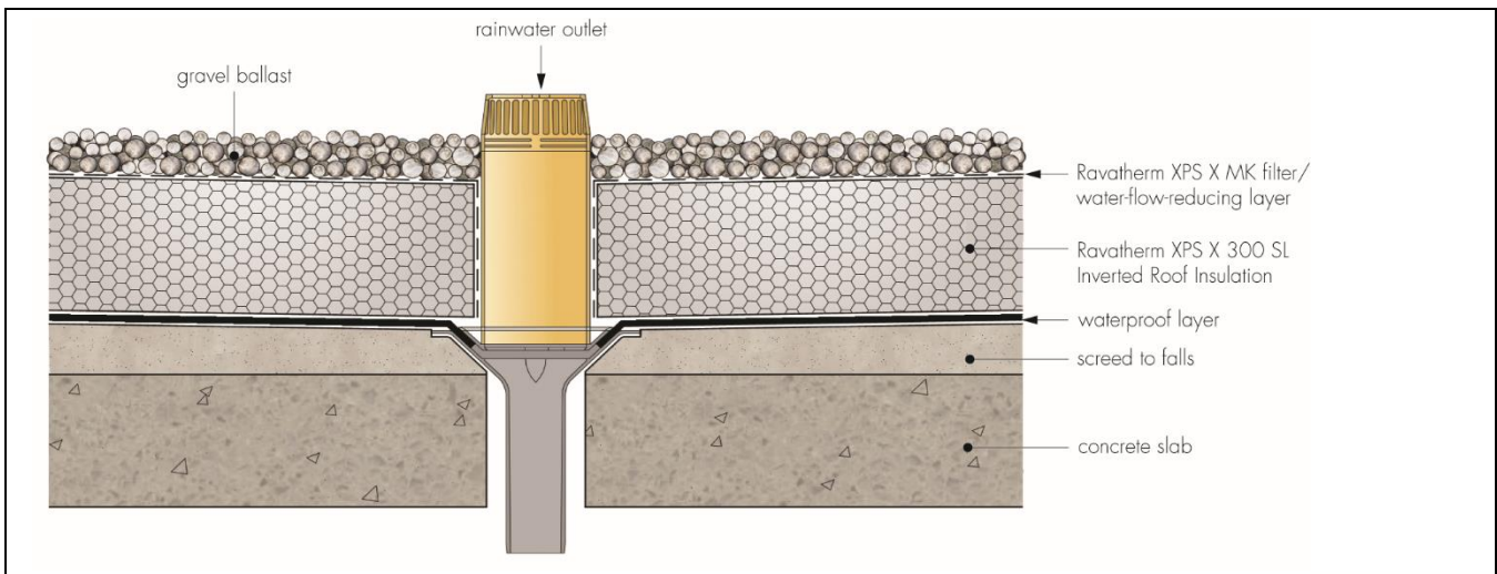
Figure 3 Water outlet detail — gravel finish
