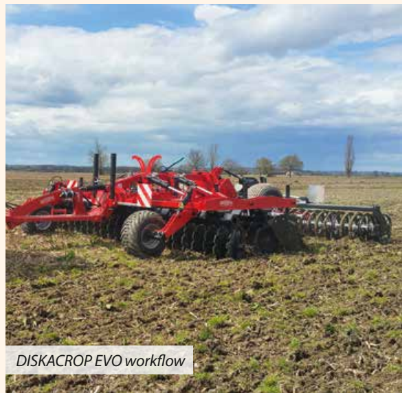
DISKACROP EVO with double U-roller, hydraulically adjustable depth wheels and nitrogen ball suspension for transport
