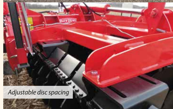
Hydraulically adjustable Z-roller Ø 500 mm, comb harrow, rear disc sections
