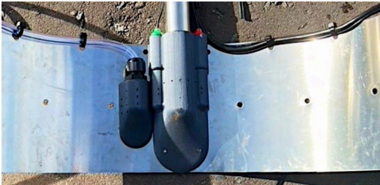
Combined NH 3 Sensor with Sampler Intake for Trade Waste, Industrial Monitoring project
