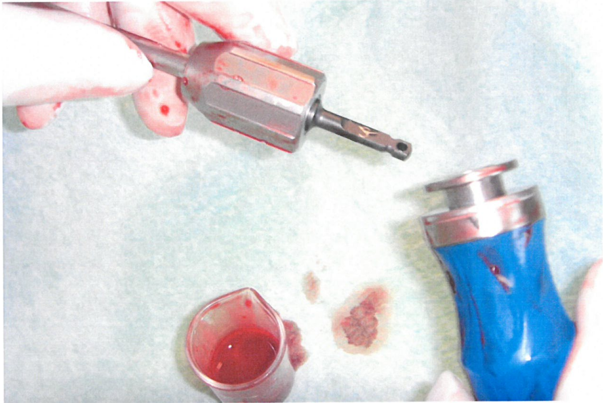
Figure 6: Contamination of an assembled sample 13616-01-1-X (X= 1, 2 and 3)
