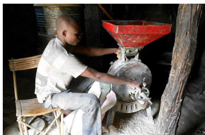
Miller using a machine running on Jatropha oil, as a substitute for diesel fuel Photo: DEM
