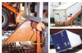
Landing gear collapse and trailer upending identified as trailer separation hazards
