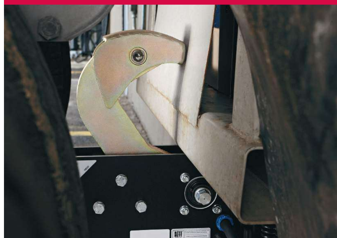
Shadow Hook Restraint with cover plate obstruction
