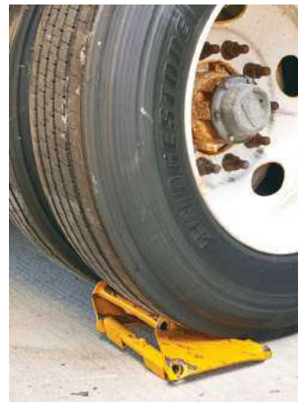
Wheel chock crushed by a truck at the loading dock
