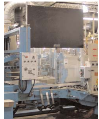
The Verti-Guard remains closed during the machine's operation, and prevents employee access.
