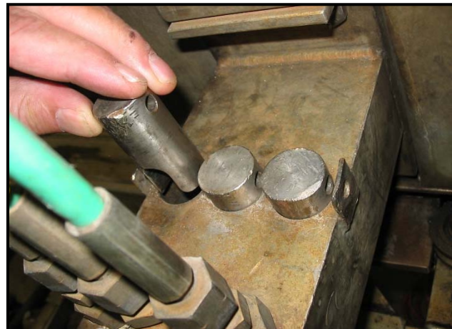
Technician Installing Hose Catcher into 3TLE Special
