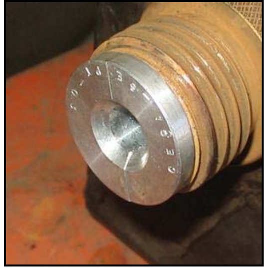
Safety Hose Catcher Mounted onto 1 LTC
