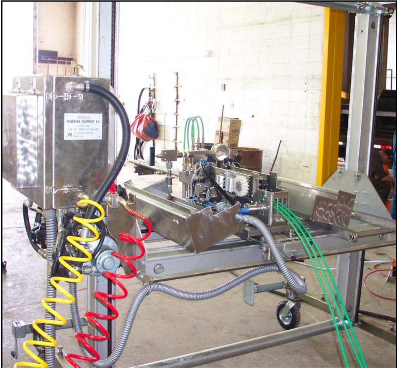
3TLE Special Installed on Positioning Frame
