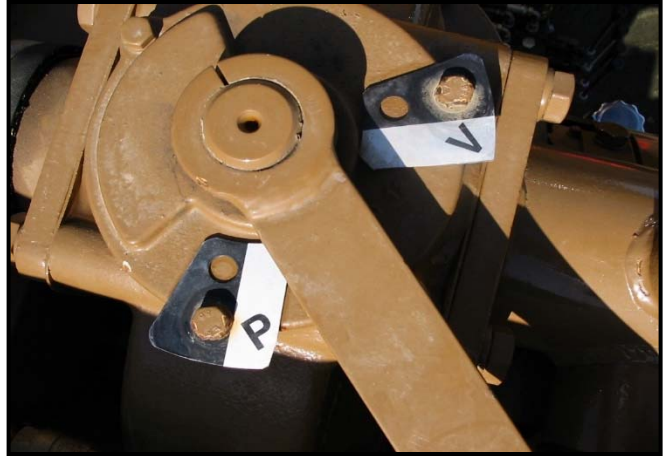
3-Way Valve in 'Neutral' Position
