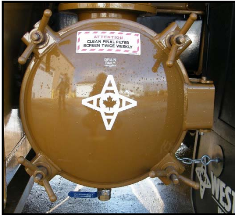
Closed Microscreen Chamber
