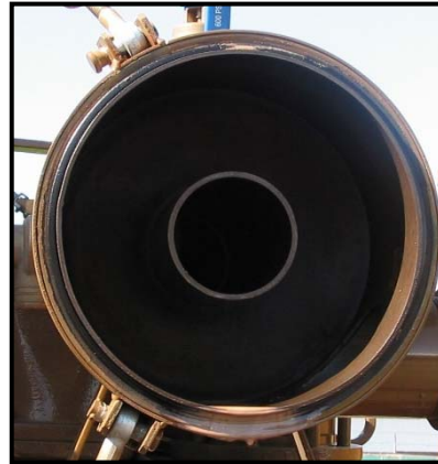
Open Microscreen Chamber
