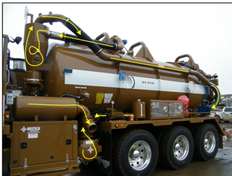
Air Flow – Negative Pressure
