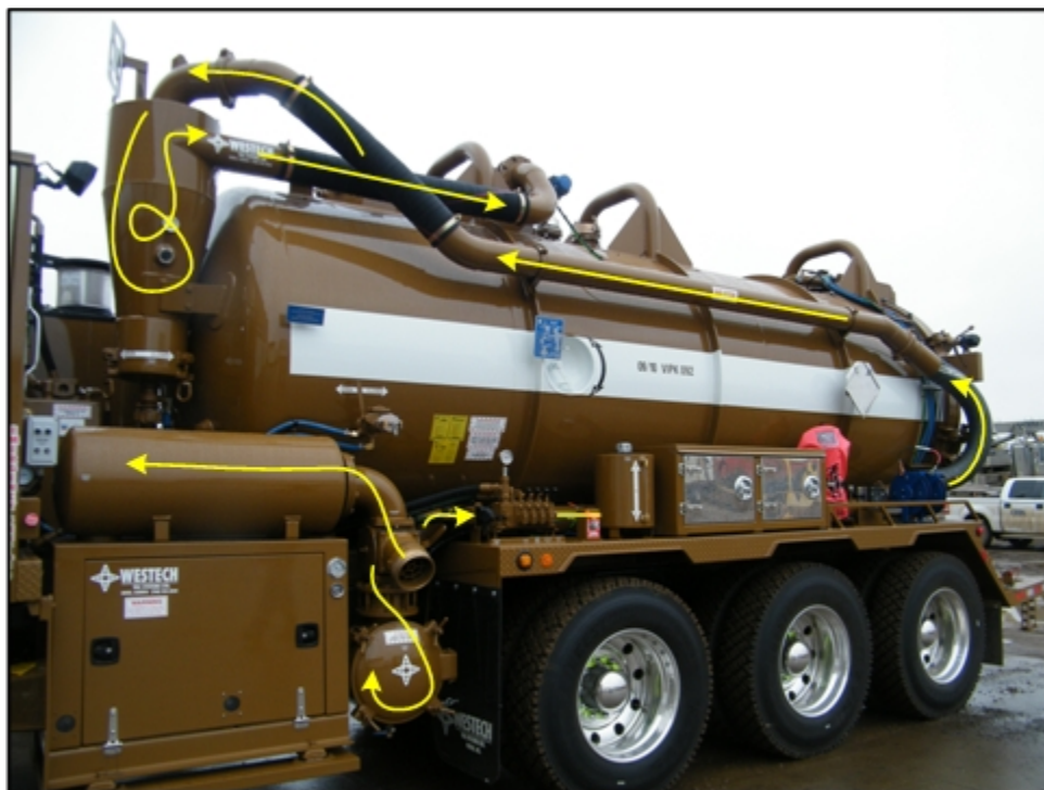
Air Flow – Positive Pressure
