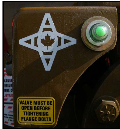
Green indicator (appears when valve in “open” position)
