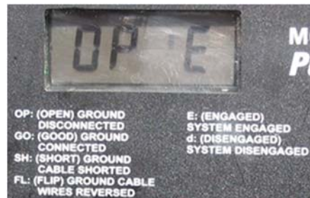
Bad (Open) Connection
