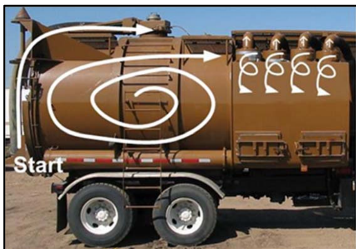
Airflow into Tank & Cyclones
