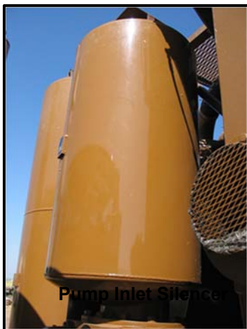
Pump Inlet Silencer
