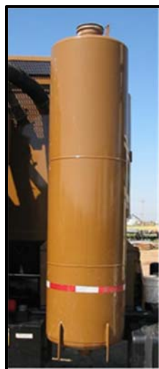
Pump Discharge Silencer
