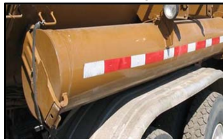
Cyclone Chamber Drain Tube
