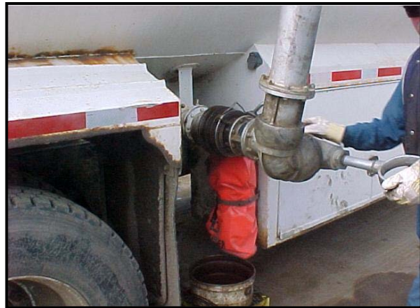
Fuel Truck Operator attaching Loading Arm to Bottom Load Connection (Simulated)
