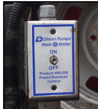
Power/ Overload Control – Close Up
