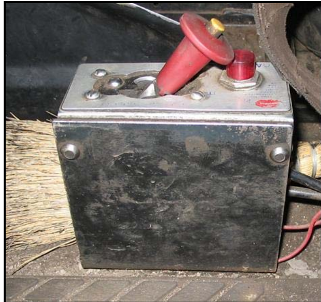
PTO Control Box
