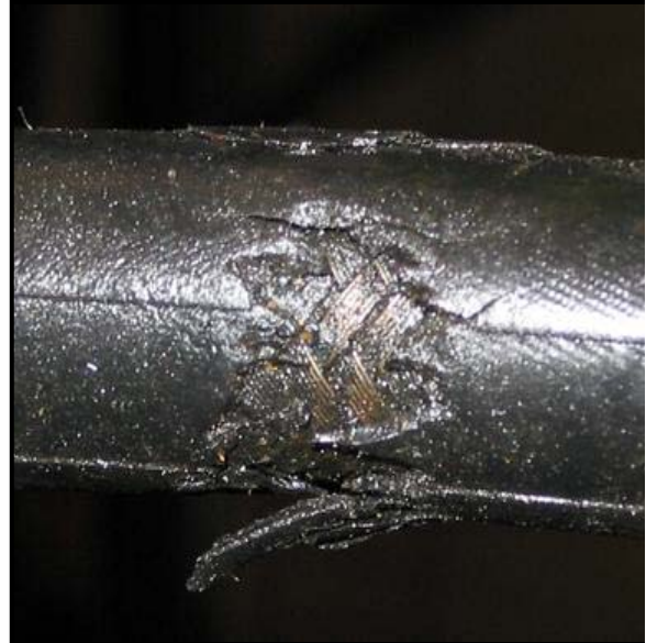
Damaged Hydraulic Lines
