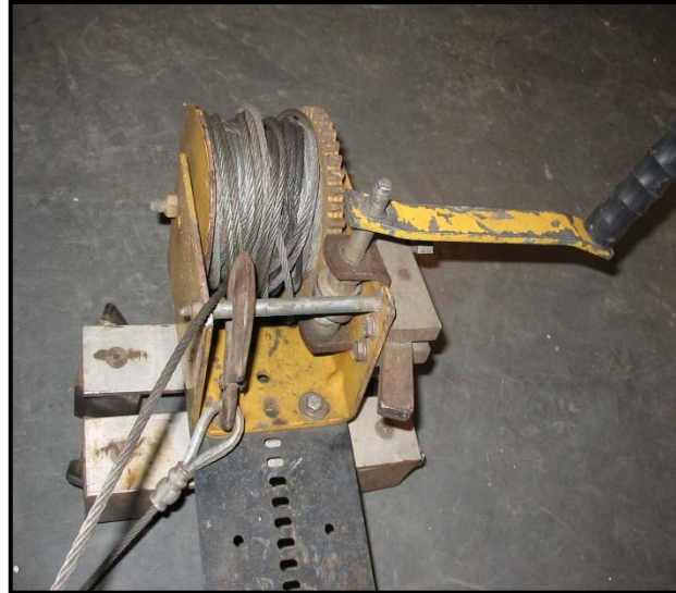
Close-up of Cable Winch Assembly
