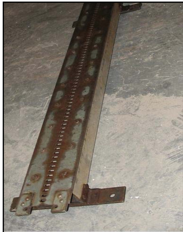
A Rigid Section of Track – Technicians will attach weights to the shoes in order to stabilize the track during concrete floor cutting operations.
