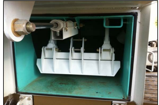
Bottom View of Mud Sweep Door (Open Position)
