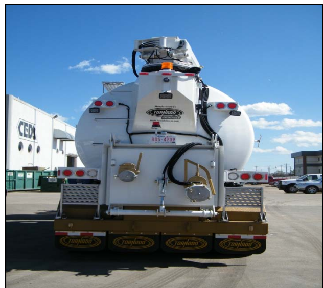
Tank Drain Valve
