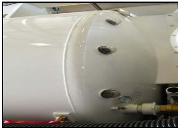
Exterior Tank Level Indicator
