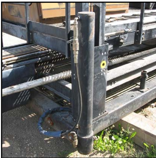
Leveling Jack used to Level Unit
