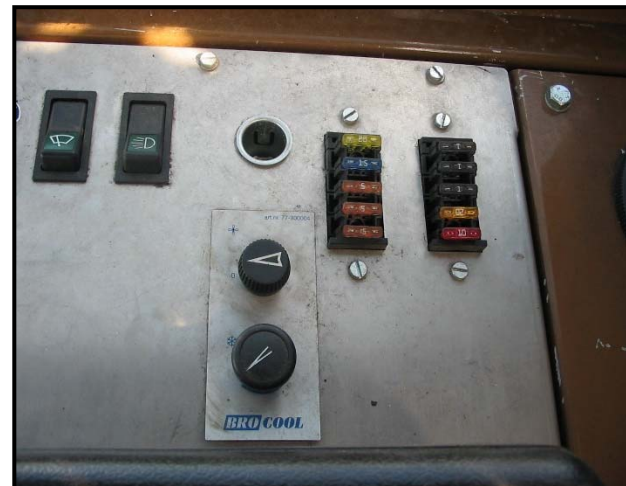
Air Conditioning Controls and Fuse Panel
