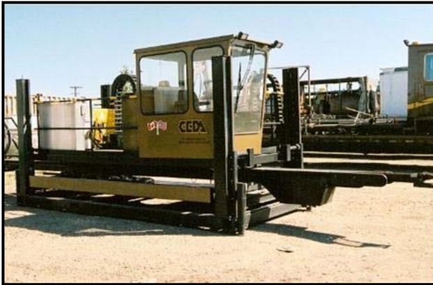
Internal Bundle Cleaner in Lowered Position
