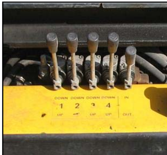
Hydraulic Bank used to Adjust Leveling Jacks
