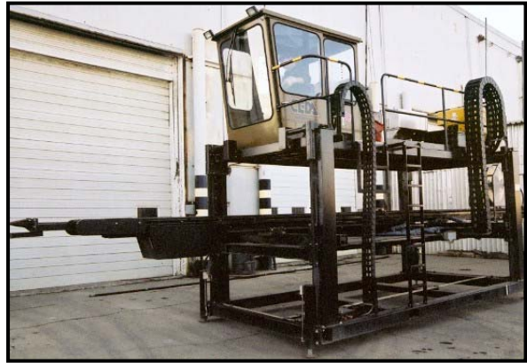
Internal Bundle Cleaner in Raised Position
