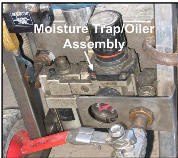
Moisture Trap / Oiler Assembly
