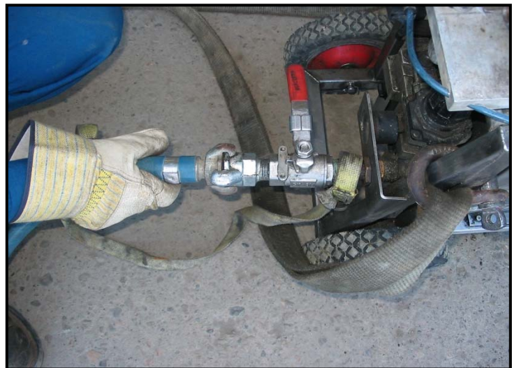
Technician Attaching Air Hose
