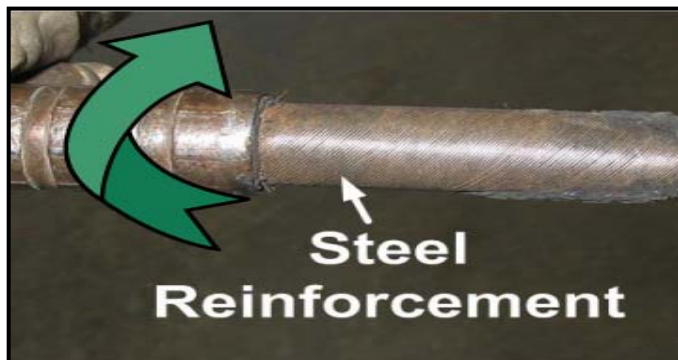
High pressure “manuli” Hose with steel braid exposed
