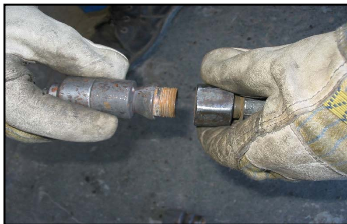
Technician Attaching a Nozzle to a high pressure hose
