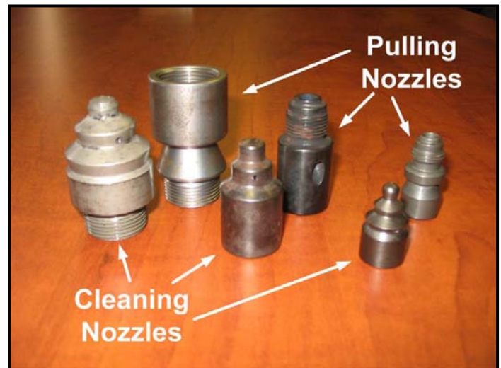
Cleaning and Pulling Nozzles. From left to right – ½", 3/8" and ¼"
