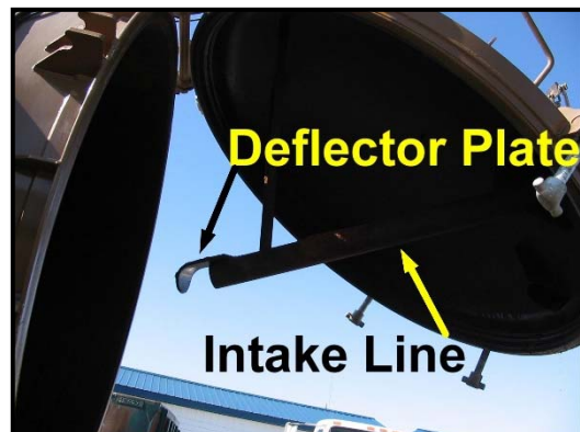
Intake Line with Deflector Plate
