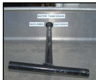
Water Tank Drain
