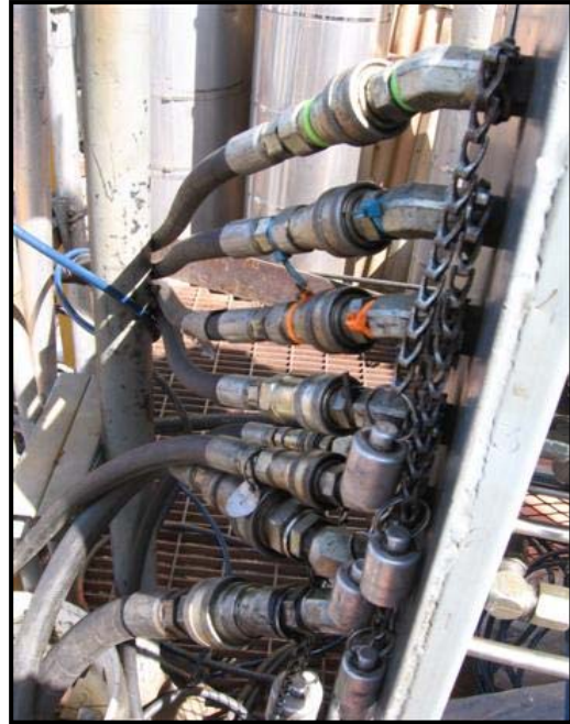
Hydraulic Hoses connect to back of Control Panel
