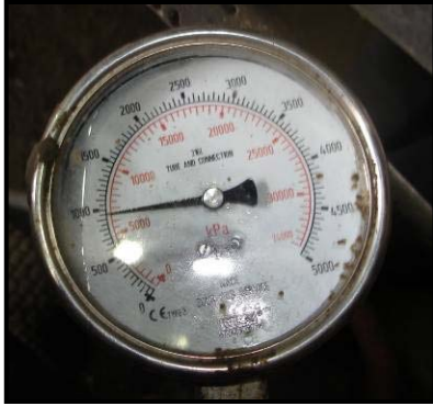
Wand Water Pressure Gauge NEVER exceed 3,000 psi
