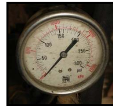
Steam Pressure Gauge NEVER exceed 150 psi
