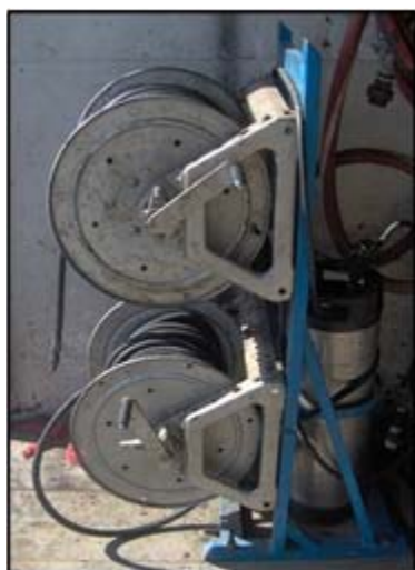
High Pressure Hose (on Hose Reels)
