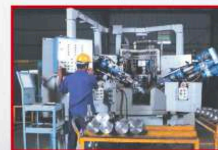
OIL HOLE DRILLING
