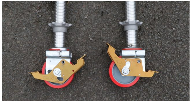
Castor locked (Note castor wheel axle has moved in line with the leg tube)
