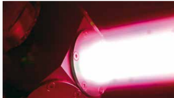
Tungsten target exposed to hydrogen plasma in the linear machine Magnum-PSI. Picture: DIFFER
