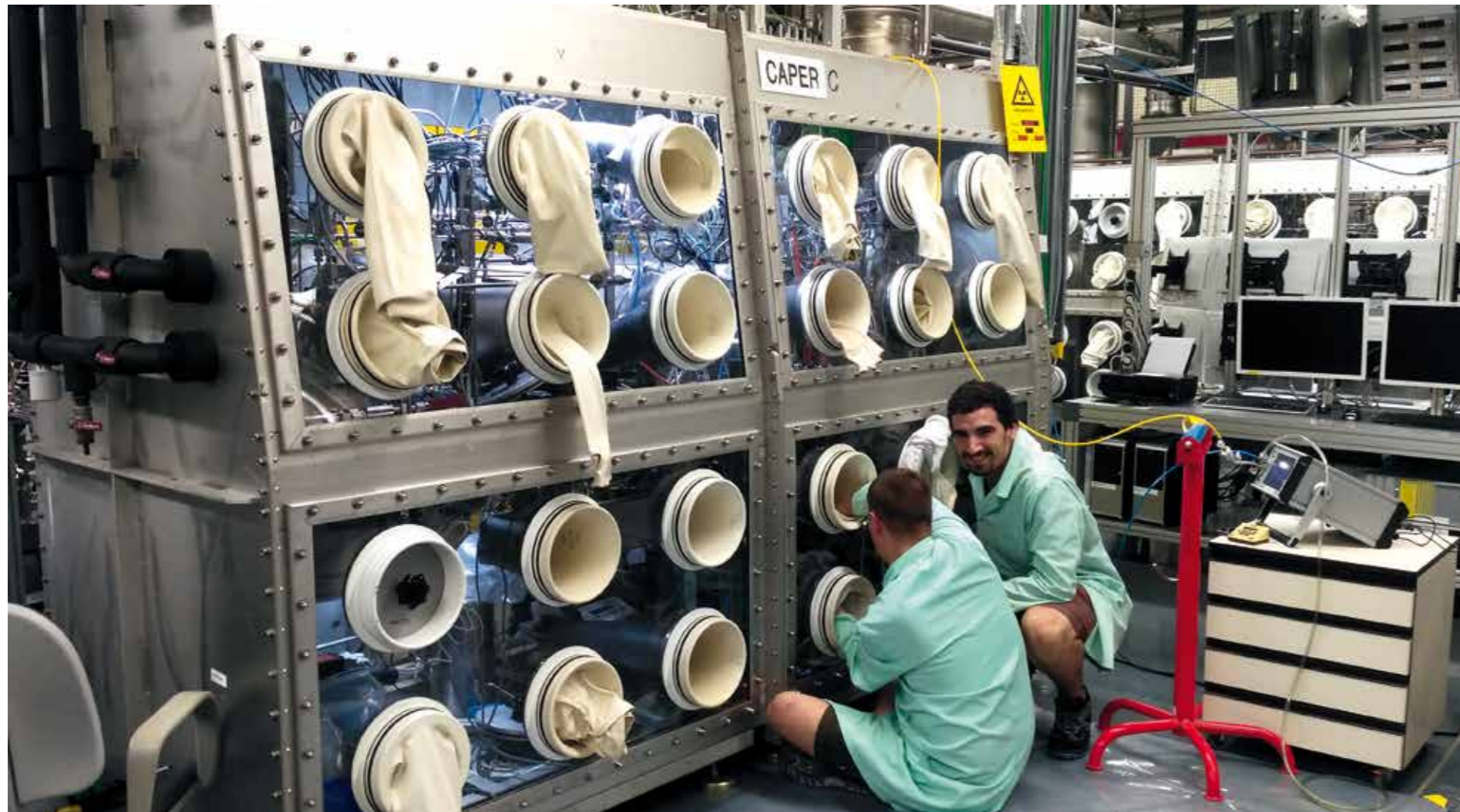
Picture 2: Rodrigo Antunes (right) and his colleague working in the “CAPER C” glovebox. This glovebox hosts the experimental setup to separate tritium species from helium with zeolite membranes, which is the core of my PhD. Picture: KIT-ITeP-TLK
