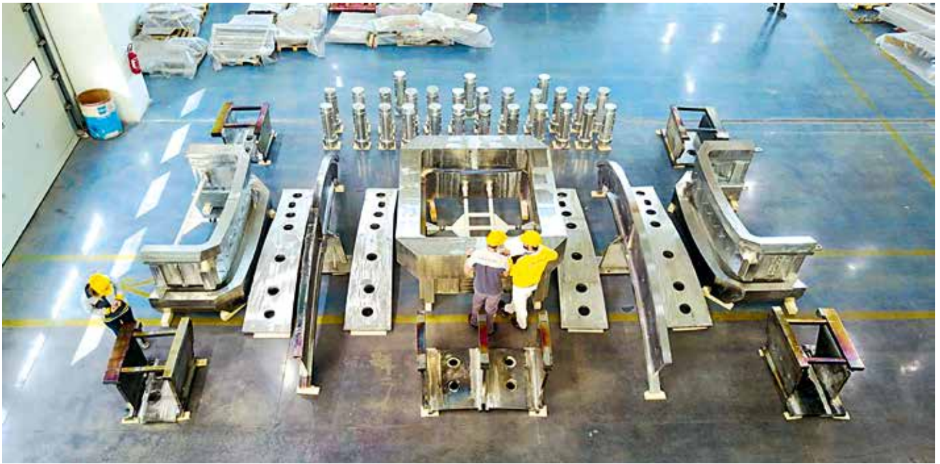
Workers place together parts of ITER's vacuum vessel at Walter Tosto. Picture: Fusion For Energy
