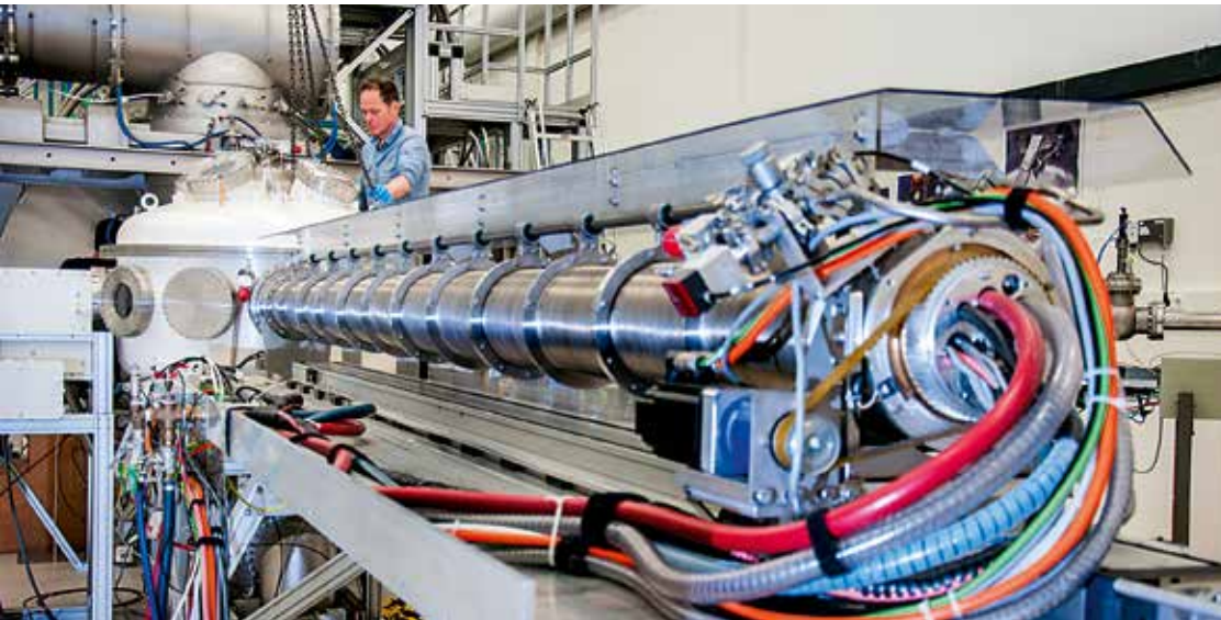
The linear plasma generator Magnum-PSI at EUROfusion's Dutch Research Unit DIFFER. Pictures: EUROfusion
