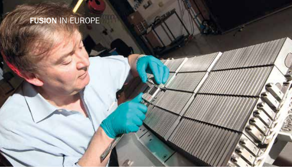
Philippe Mertens from Forschungszentrum Juelich is checking the solid tungsten lamellae on a divertor. The divertor is deals with immense heat loads in fusion experiments. Picture: EUROfusion
