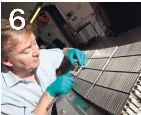
6 Philippe Mertens (FZ Juelich) is checking a divertor. Heat exhaust systems play a major role in EUROfusion's programme. Picture: EUROfusion
