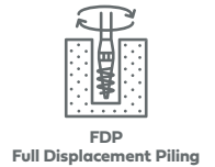
FDP Full Displacement Piling
