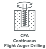
CFA Continuous Flight Auger Drilling
