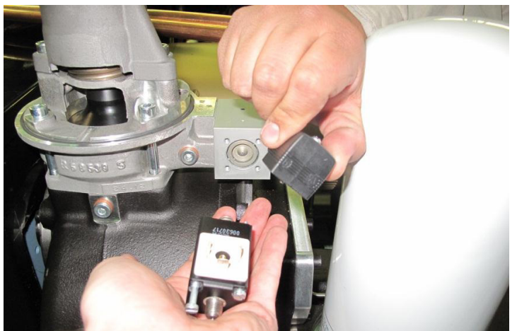
Electrical connection removed
