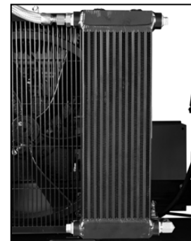
Air cooled after cooler on Platinum models
