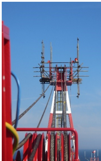
Photo: New crane boom tip
