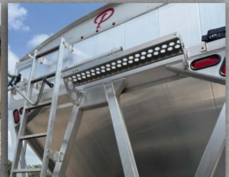
Easy access ladders & catwalks
