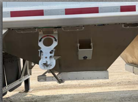
Self locking chute opener & hammer hit bracket
