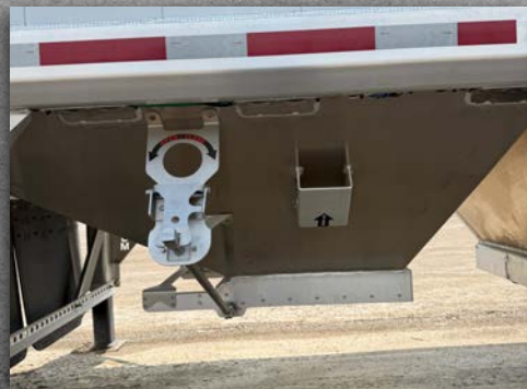
Self locking chute opener & hammer hit bracket
