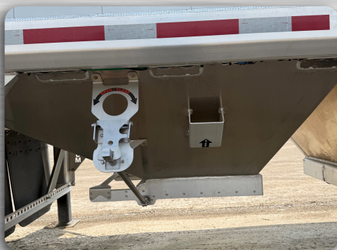
Self-locking chute opener & hammer hit bracket
