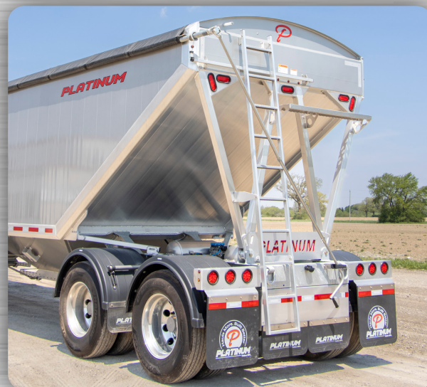
Heavy duty aluminum tarp bows & vented mid wall
