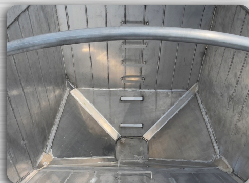
Heavy duty aluminum tarp bows & vented mid wall
