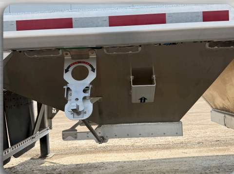
Self-locking chute opener & hammer hit bracket
