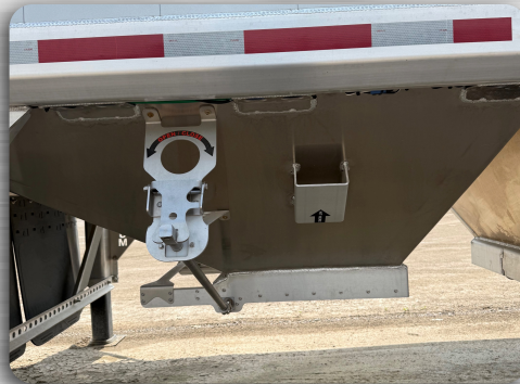
Self-locking chute opener & hammer hit bracket
