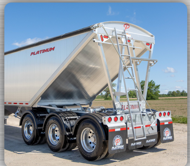
Heavy duty aluminum tarp bows & vented mid wall
