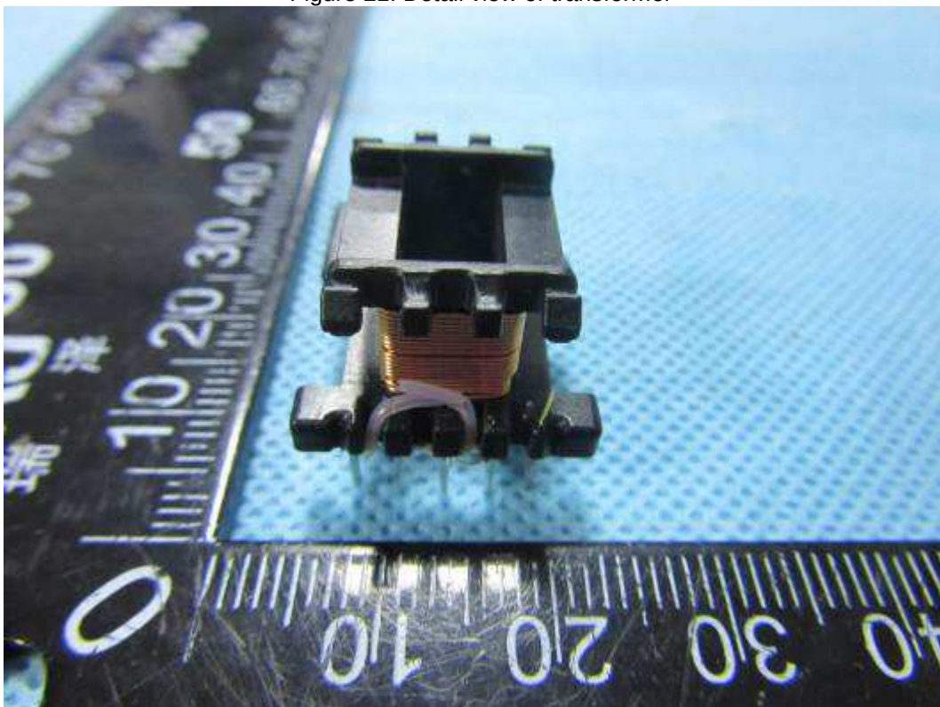
Figure 22. Detail view of transformer
