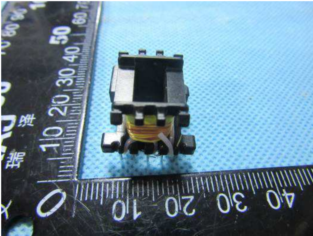
Figure 21. Detail view of transformer
