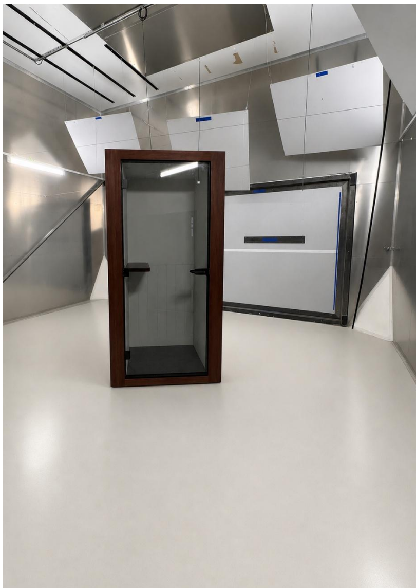
Figure 3 – XF Classic Booth in reverberation room (first position)
