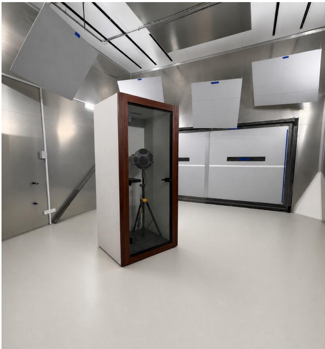
Figure 4 – XF Classic Booth in reverberation room (second position)
