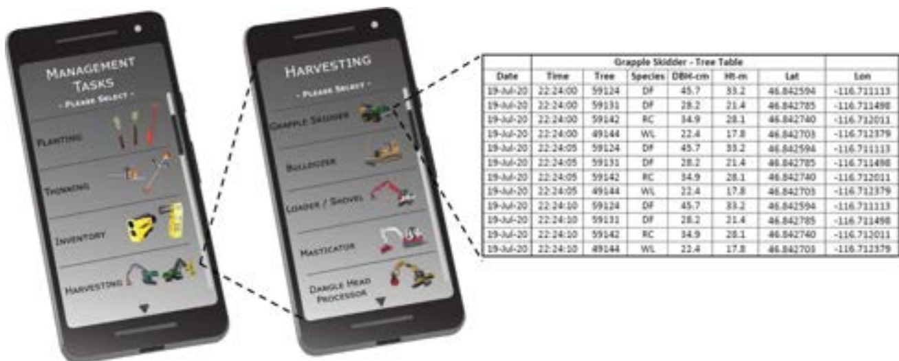
Fig. 4 Conceptual mobile application framework for maintaining individual motor-manual worker and equipment activity recognition information coupled with individual tree and product data in a networked, relational database at the jobsite. Tables are associated with
