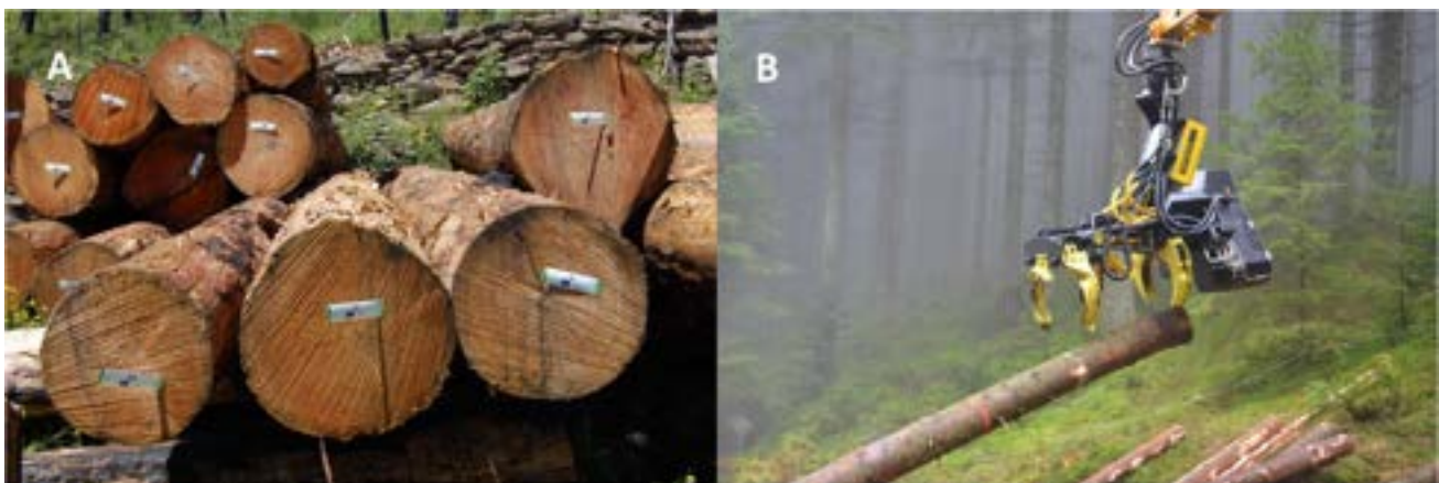
Fig. 3 A RFID tags on log ends for stump-to-mill traceability tests in the Italian Alps (Trento), B sensorized processor head described in Sandak et al. [75••] featuring log-grading sensors (i.e., timber den-
