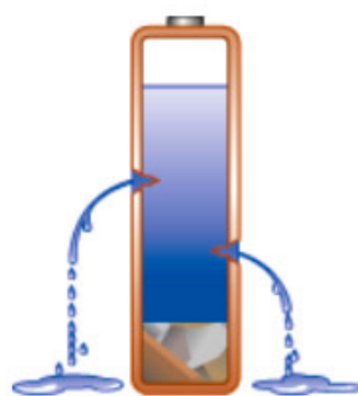
Figure 6: Effects of high self-discharge
