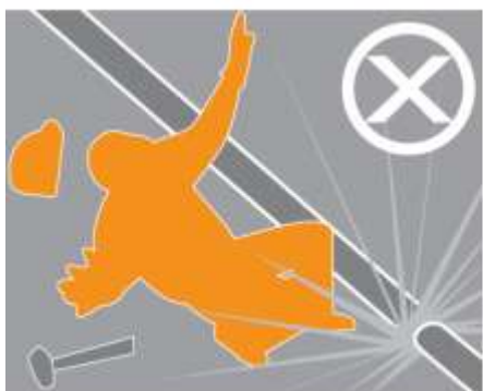
Never dismantle pipeline while under pressure
