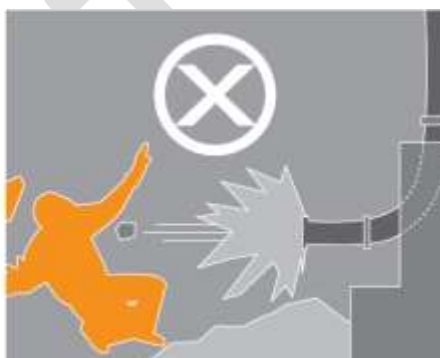
Keep clear of discharge end of pipe
