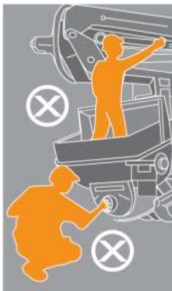
Dangerous cleaning practices
