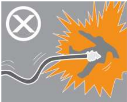
End-hose should be secured or removed
