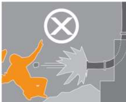
Keep clear of discharge end of pipe
