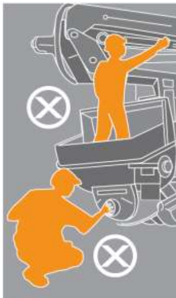
Dangerous cleaning practices
