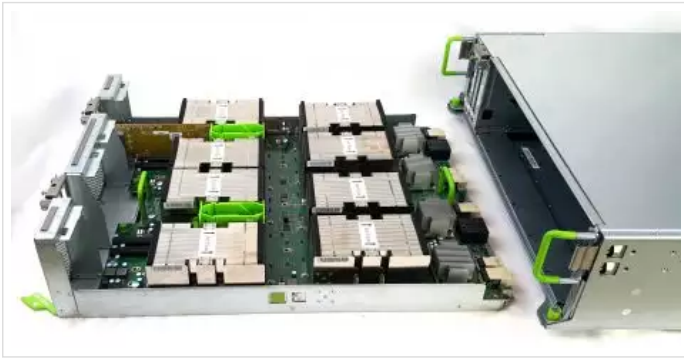
Big Basin, Facebook's latest AI server. Each of the eight heat sinks hides a GPU. (Photo: Facebook)
