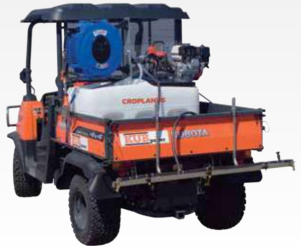
MC6 FIREBREAK BOOM SHOWN FITTED TO TRAY
