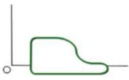
Worn or cracked pump
