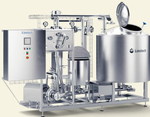
Upgraded: CIP Dosing and reuse water unit
