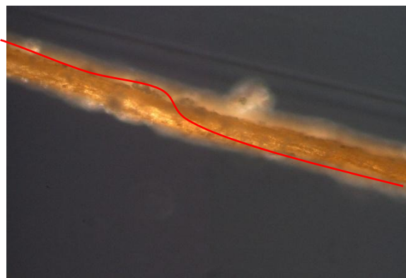
Figure 16 Single fiber strand under 20x transmitted light
