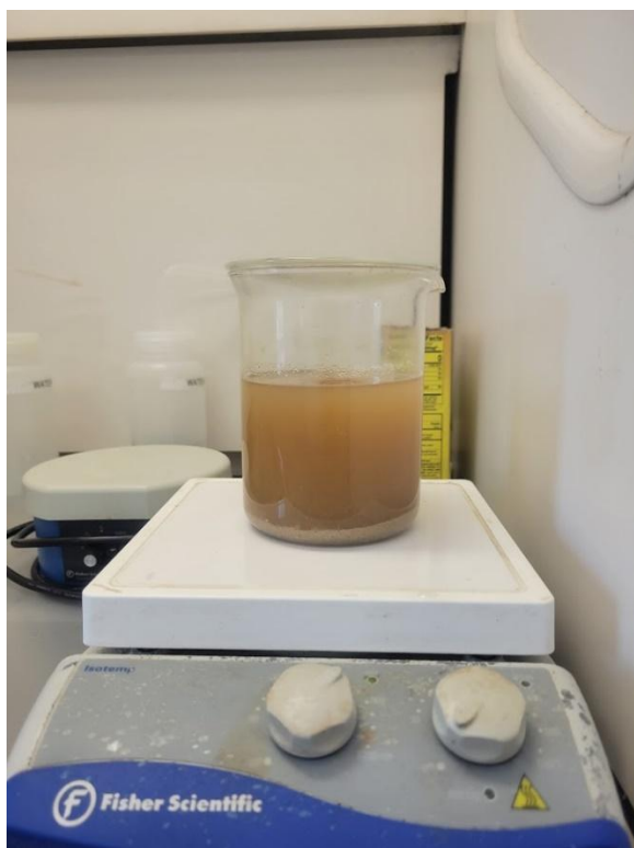
Figure 8 Sample HC-01 During Acid Digestion
