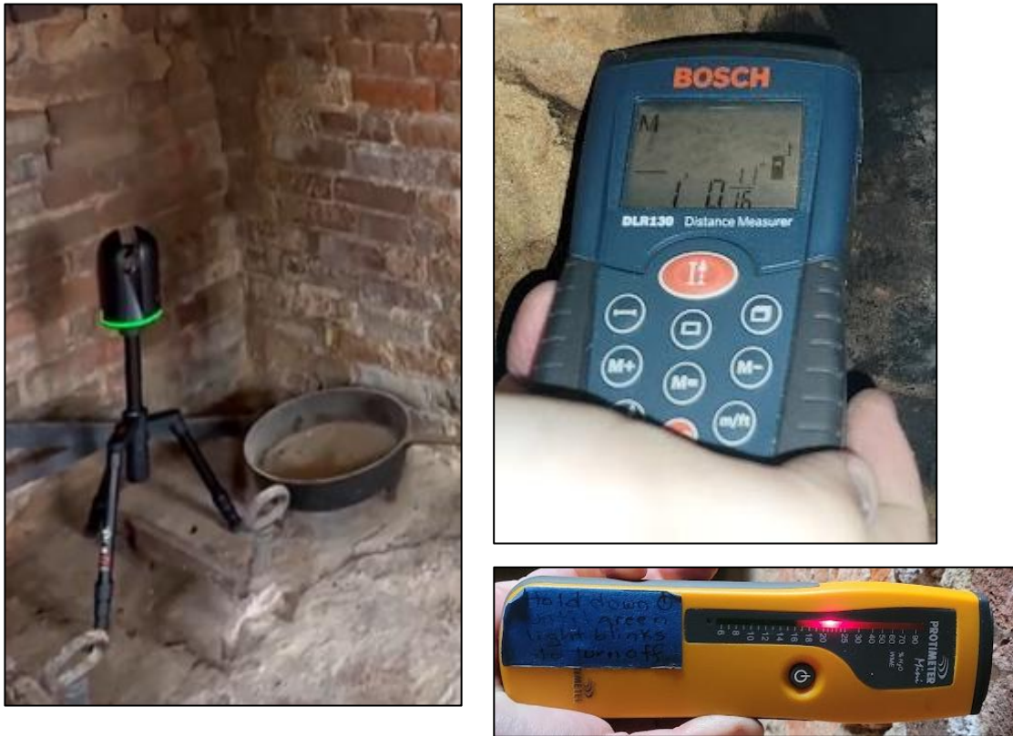
Figure 4 Tools Used. Showing the Laser Scanner, Laser Tape, and Moisture Meter
