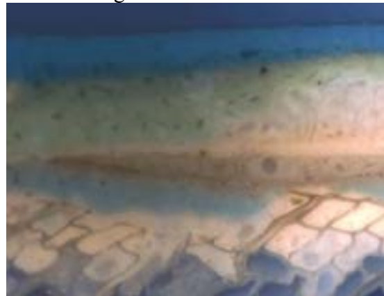
Room 102 Comparative Paint Stratigraphies on the Cupboard, Paneling, Doors and Trim
