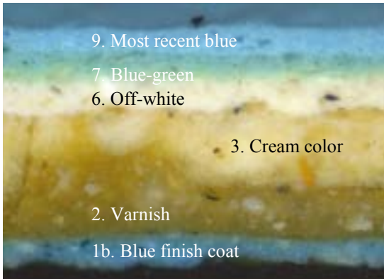
102-17. Architrave for original west door. Visible Light 200X
