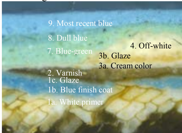
Room 102 Comparative Paint Stratigraphies on the Cupboard, Paneling, Doors and Trim
