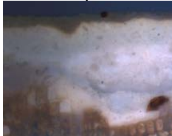
Room 104 Comparative Paint Stratigraphies on the Window Trim, Cupboard and Boards
