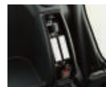
Central fuse box located behind seat
