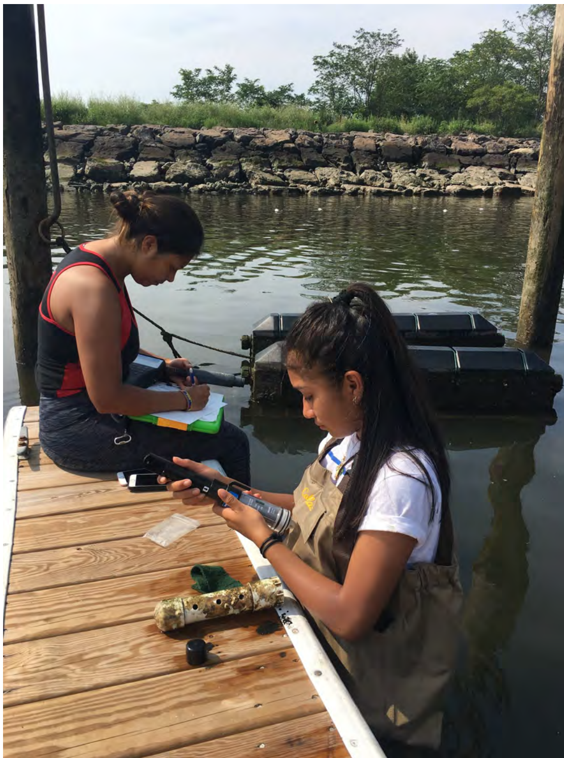
Figure 19. TNC Marine Science Technician Tatiana Castro-Gallego and Billion Oyster Project Summer Intern Lisette Mejia monitor water quality with HORIBA water quality meters and maintain HOBOT logger equipment. (Photo courtesy of Elizabeth Burmester)
