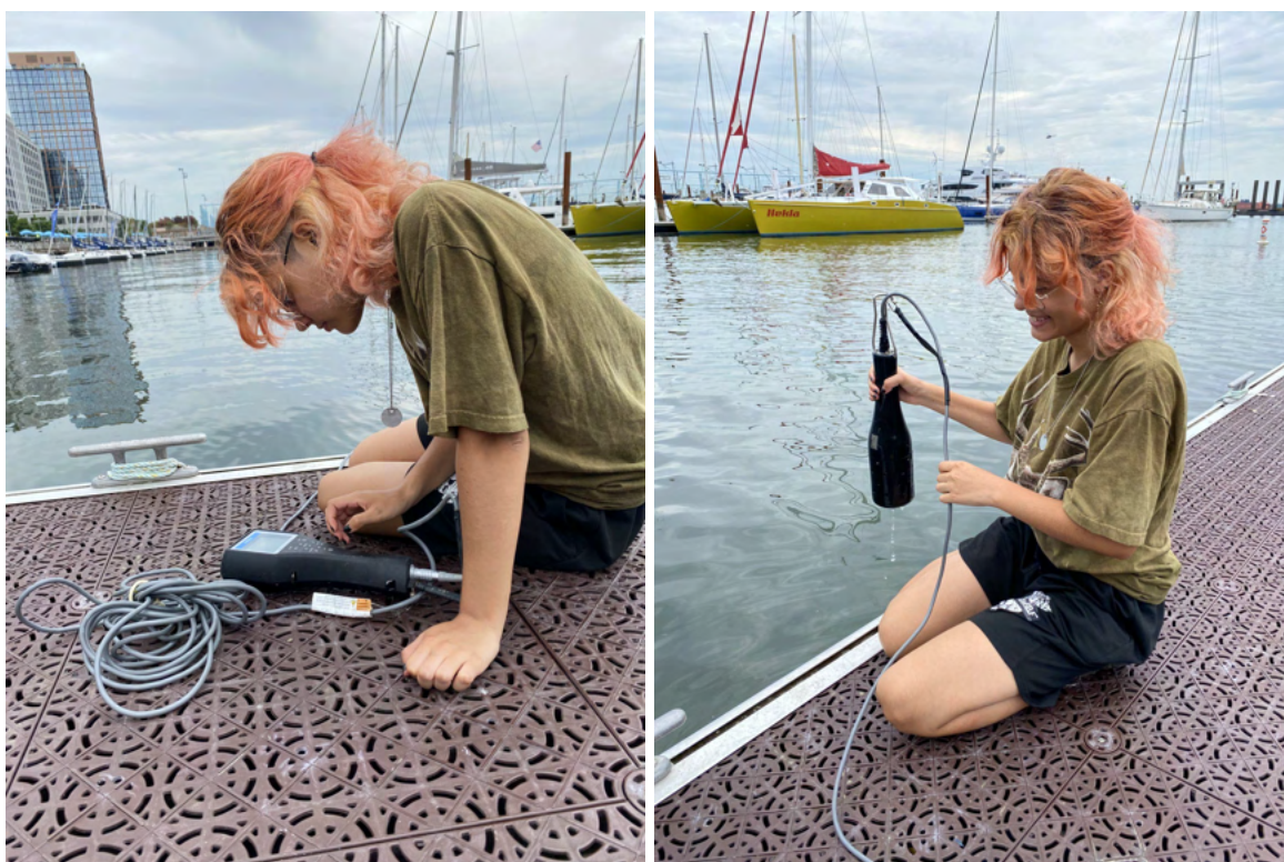
Figure 28. Billion Oyster Project summer intern deploying the Horiba probe at Brooklyn Bridge Park One°15 Brooklyn Marina (right) and recording point water quality measurements using the Horiba hand-held device (left). (Photos courtesy of Jennifer Zhu)
