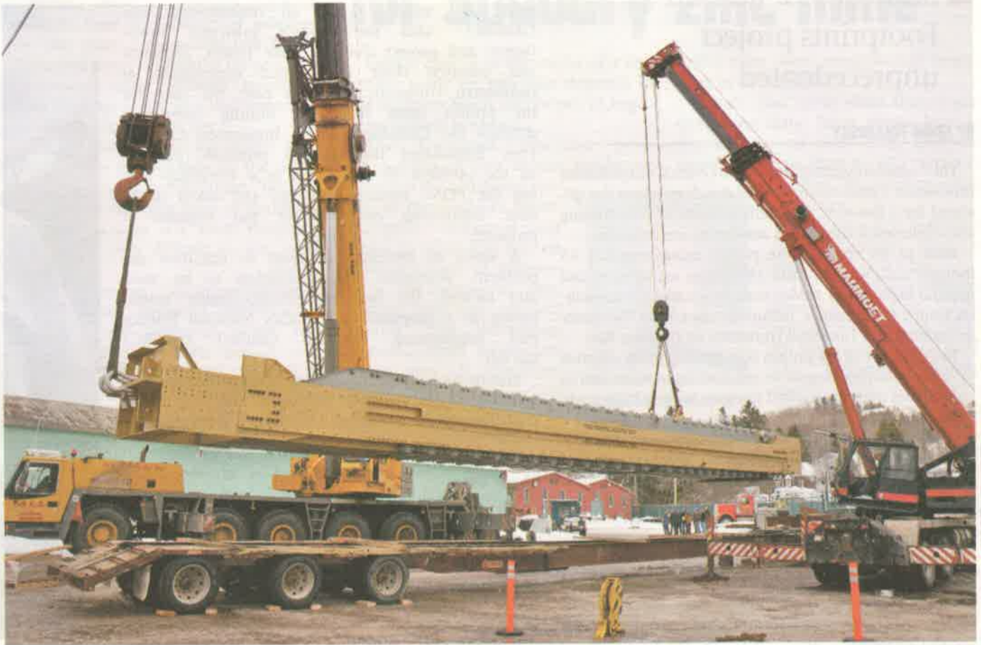
Made of welded steel, each 68-foot high skip is capable of hoisting potash at 4,000 feet-per-minute in the 3,600-foot Vanscoy shaft.
